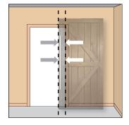
To position Wall Mount properly, place it slightly overlapping the wall opening. For this setup, ensure your door width meets these criteria: Subtract the desired coverage (e.g., 6") from the opening width 7-3/4". For instance, with a 40-inch wall opening, your minimum door width should be 41.5 inches. In this case, a standard 42-inch-wide door is recommended.
