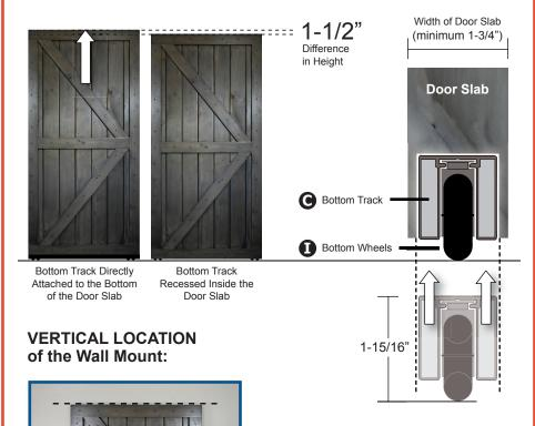
To figure out exactly how high the Wall Mount should be installed on the wall, lift the Door Slab up and position as closely as you can to the wall. This step may require two people to perform. See page 14 for further information.
