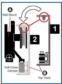
Slowly lower the door, making sure that the grooved wheel on the Wall Mount fits inside the Top Track Channel and, at the same time, the Bottom Track is lowered over the Door Floor Guide.
