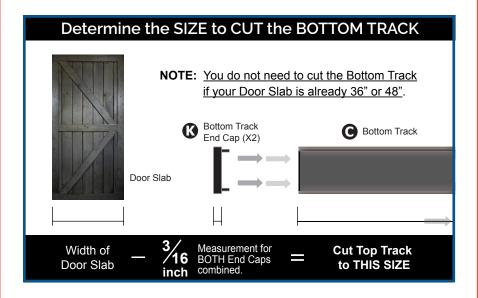
By subtracting the width of **BOTH** End Caps from the width of the Door Slab (3/16"), this will allow the **Bottom Track to be flush at both ends** after installation with both End Caps attached..
