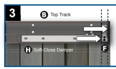
Once the End Cap is secured, slide the Hard Stop all the way over <u>flush</u> with the End Cap. Tighten Built-In Screws to secure. Slide the Soft-Close all the way over <u>flush</u> with the <u>Hard Stop</u>. Tighten screws to secure.
