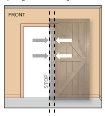
A **Partially Open** door that stops short of being flush from the wall opening allows a person to grab the door to open or close.
