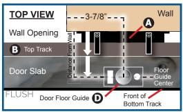
$$\left(1\frac{9^{n}}{16} + \frac{Door}{Thickness}\right) - \left(\frac{11^{n}}{16}\right) = \frac{Distance}{From Wall}$$
