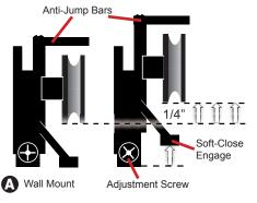
and should not be altered in any manner. If the slab moves smoothly in the open and closed positions then no adjustment is needed. Turning the screw clockwise raises the roller assembly. Adjust the roller assembly as needed until the door moves smoothly in both the open and closed positions.
